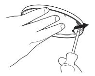
3. Fit Your FireAngel® Smoke Alarm Hold the alarm up to the base plate and push and rotate the alarm clockwise into position as shown. Make sure that the unit is securely fitted.
